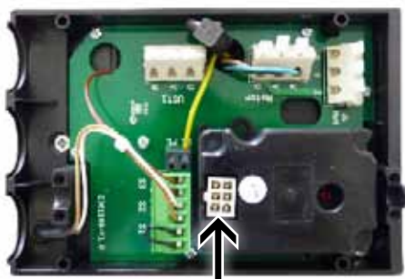
Six-pole plug Control unit connection cable
