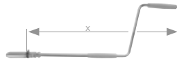
24 334.0701 Crank handle with universal joint for D.M and W.M drives x = 1.35 \text{ m}
